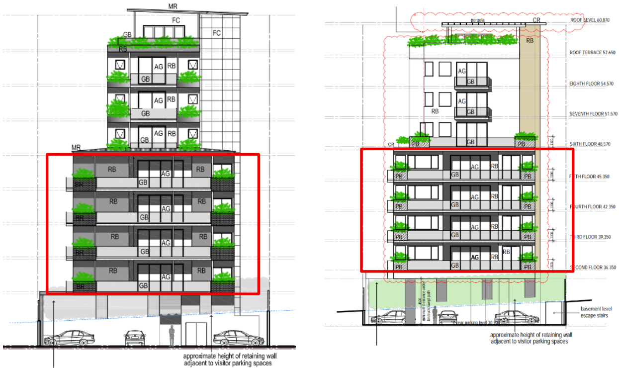
Figure 4 Originally Approved Rear Exterior Levels 2-5 (Left), Proposed Rear Exterior Changes Levels 2-5 (Right)
