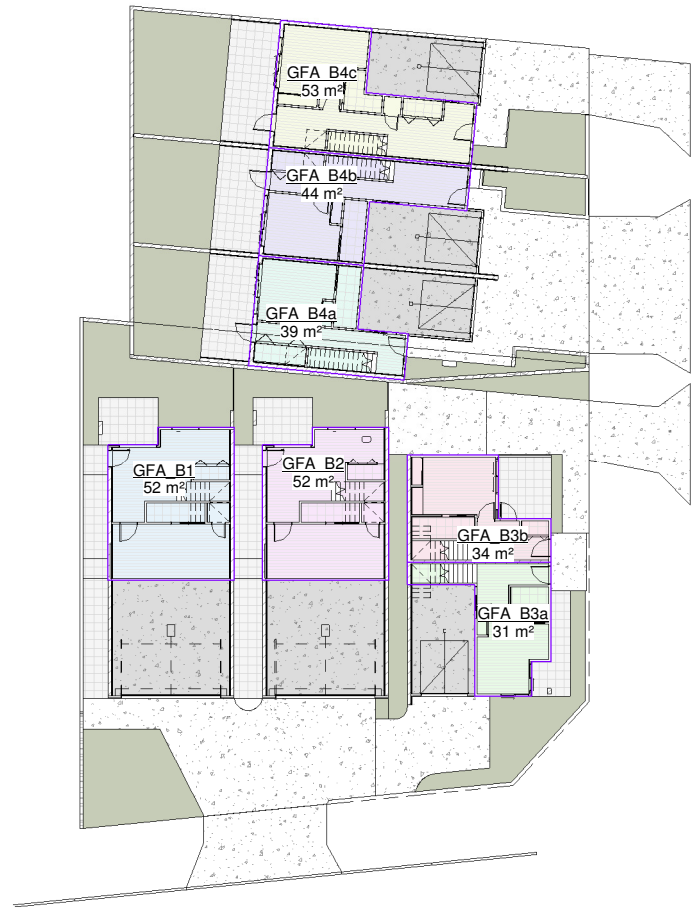
1 GROUND FLOOR 1 : 200 on A1 / 1 : 400 on A3
