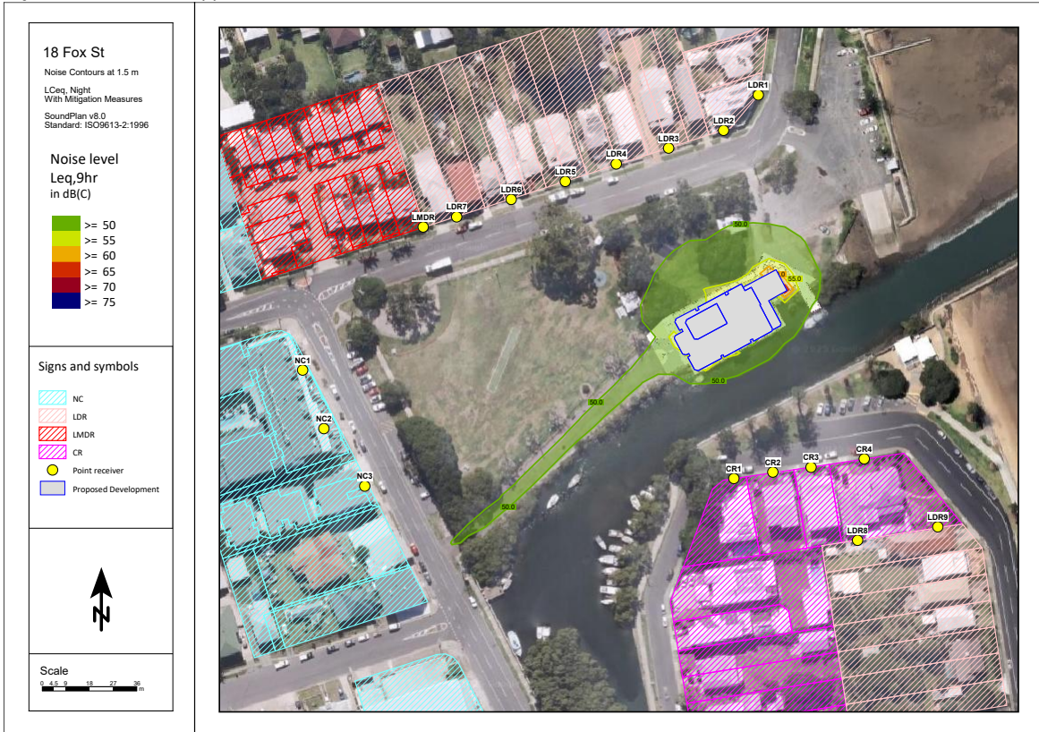
Plate B18: Noise contours at 1.5m above ground, L eq night with mitigation measures . Levels are in dB(C) and include façade effects where applicable.
