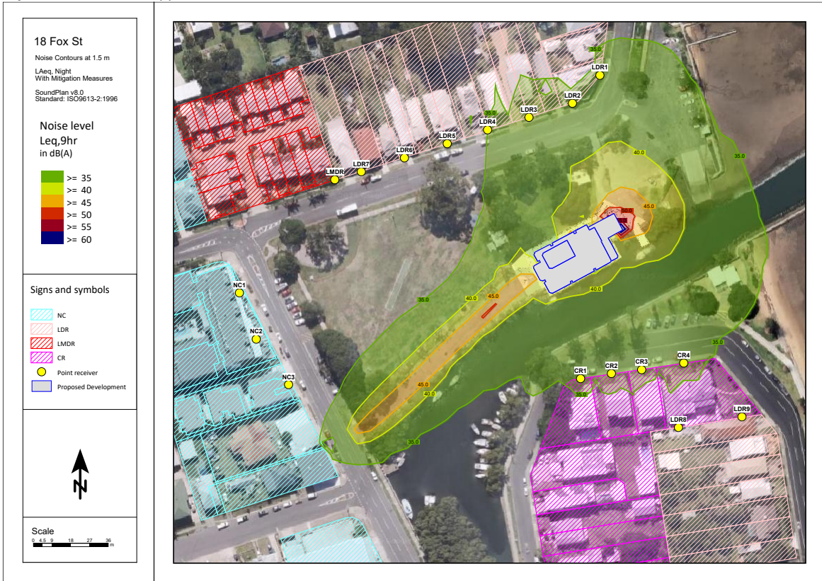
Plate B15: Noise contours at 1.5m above ground, LAeq night with mitigation measures . Levels are in dB(A) and include façade effects where applicable.
