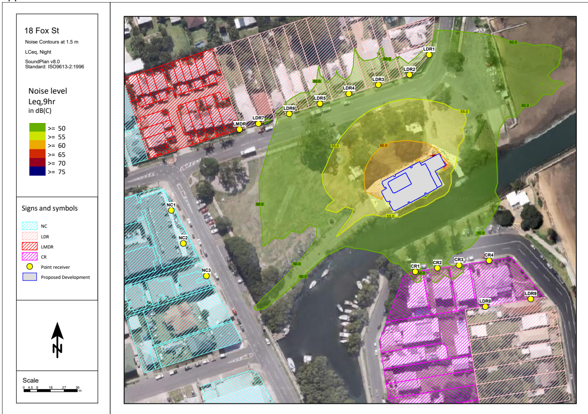
Plate B11: Noise contours at 1.5m above ground, L Ceq night. Levels are in dB(C) and include façade effects where applicable.
