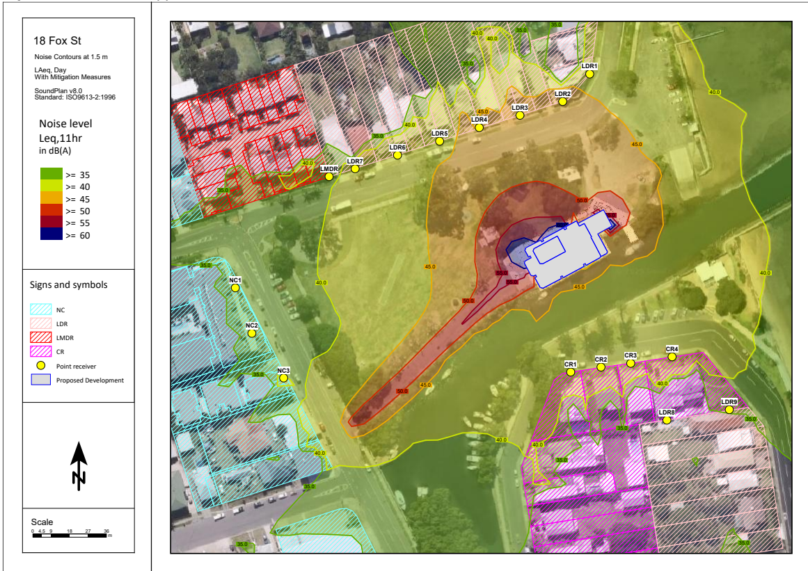
Plate B13: Noise contours at 1.5m above ground, LAeq day with mitigation measures . Levels are in dB(A) and include façade effects where applicable.
