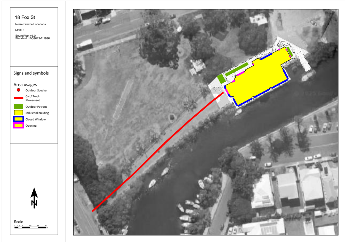
Plate B1: Location of noise sources, Level 1 (zoomed out to show vehicle movements).
