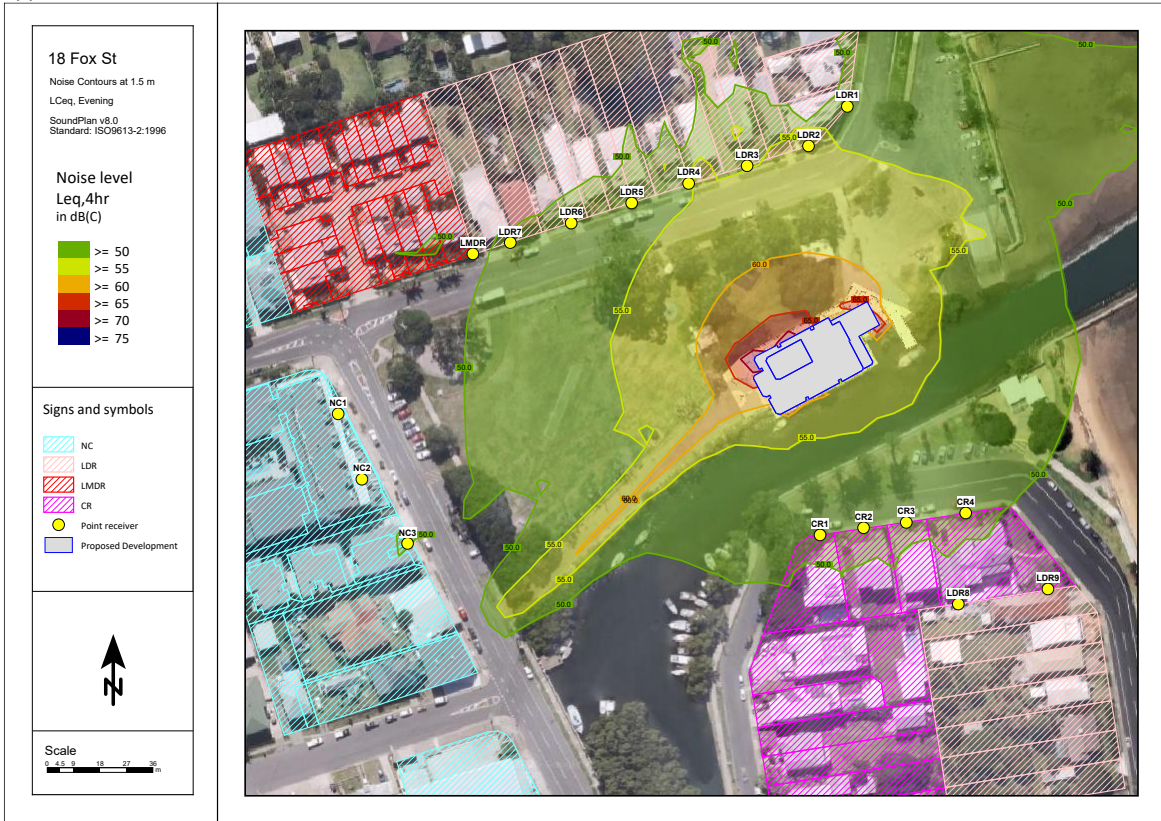
Plate B10: Noise contours at 1.5m above ground, L Ceq evening. Levels are in dB(C) and include façade effects where applicable.
