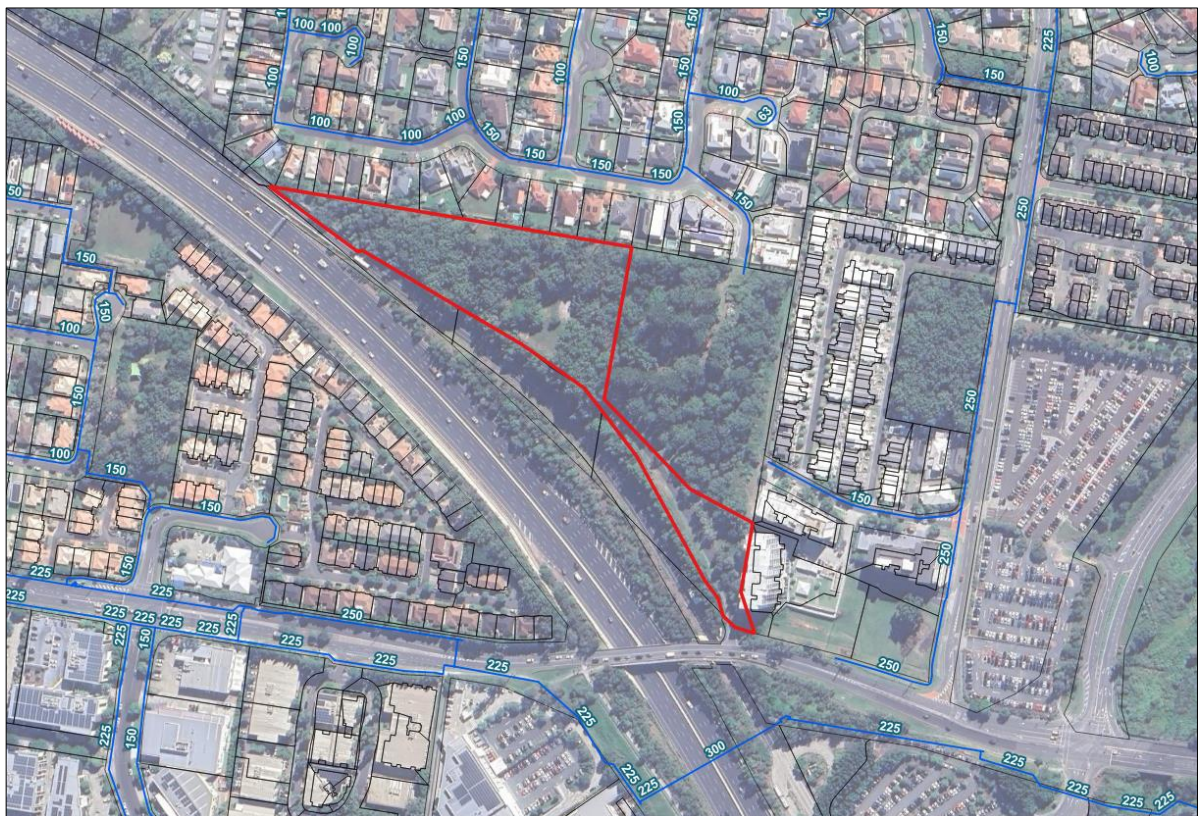
Figure 5-2 – Existing Water Reticulation Main (QLD Urban Utilities)
