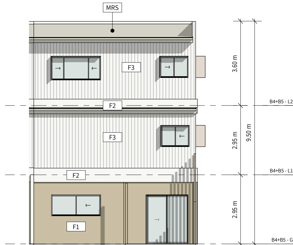
A UNIT TYPE 3 ELEVATION 1:100 @ A3
