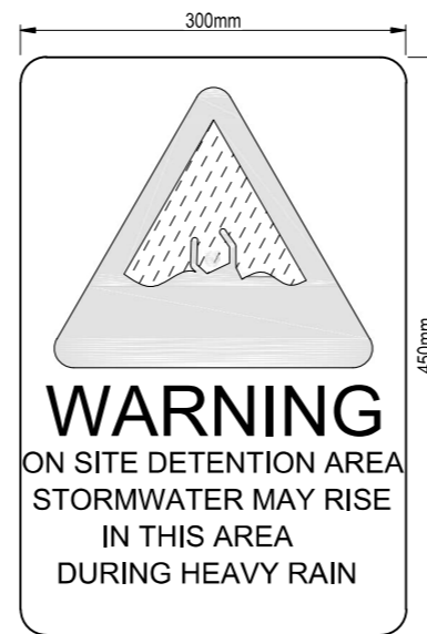
ON SITE STORMWATER DETENTION WARING SIGN
