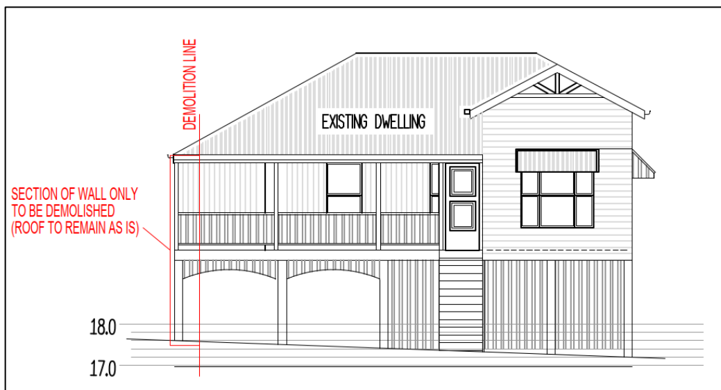
Figure 4 – Proposed demolition (front)
