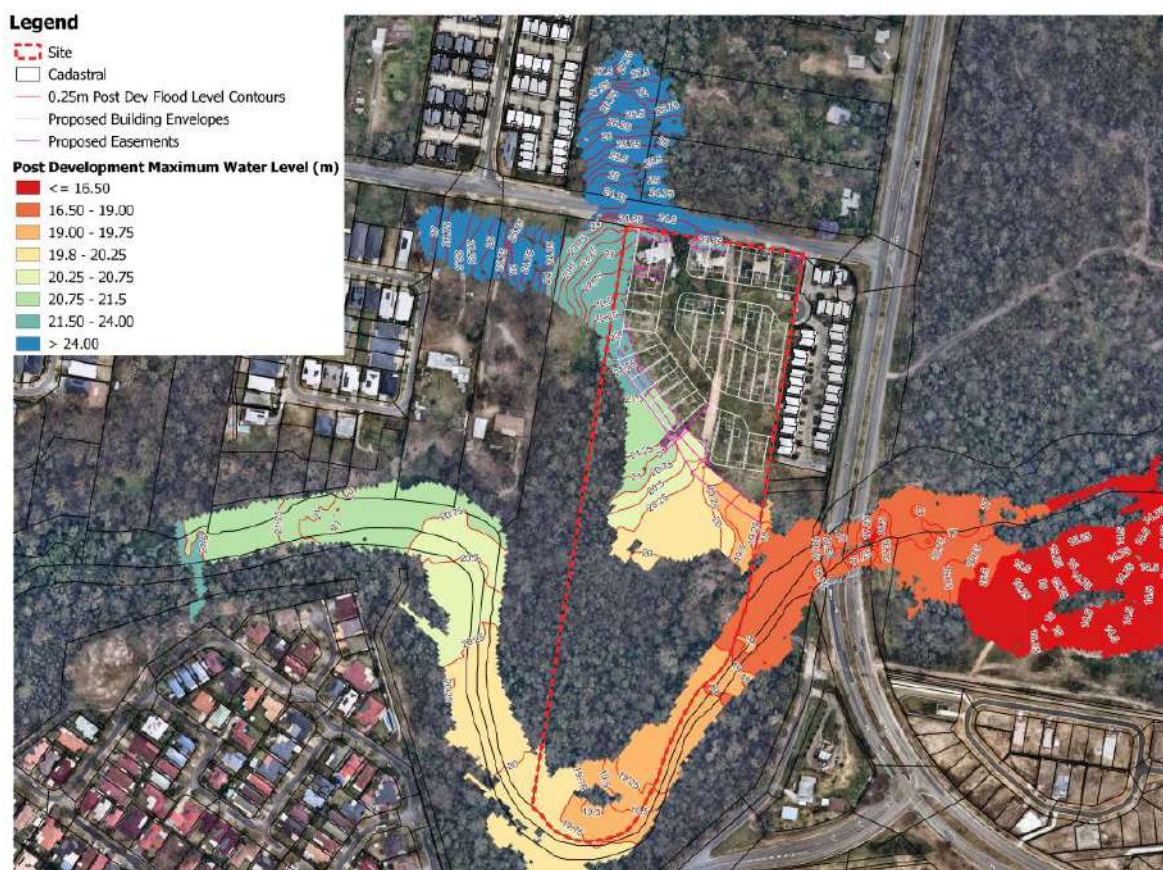
Figure 10: 2% AEP Post Development Flood Levels
