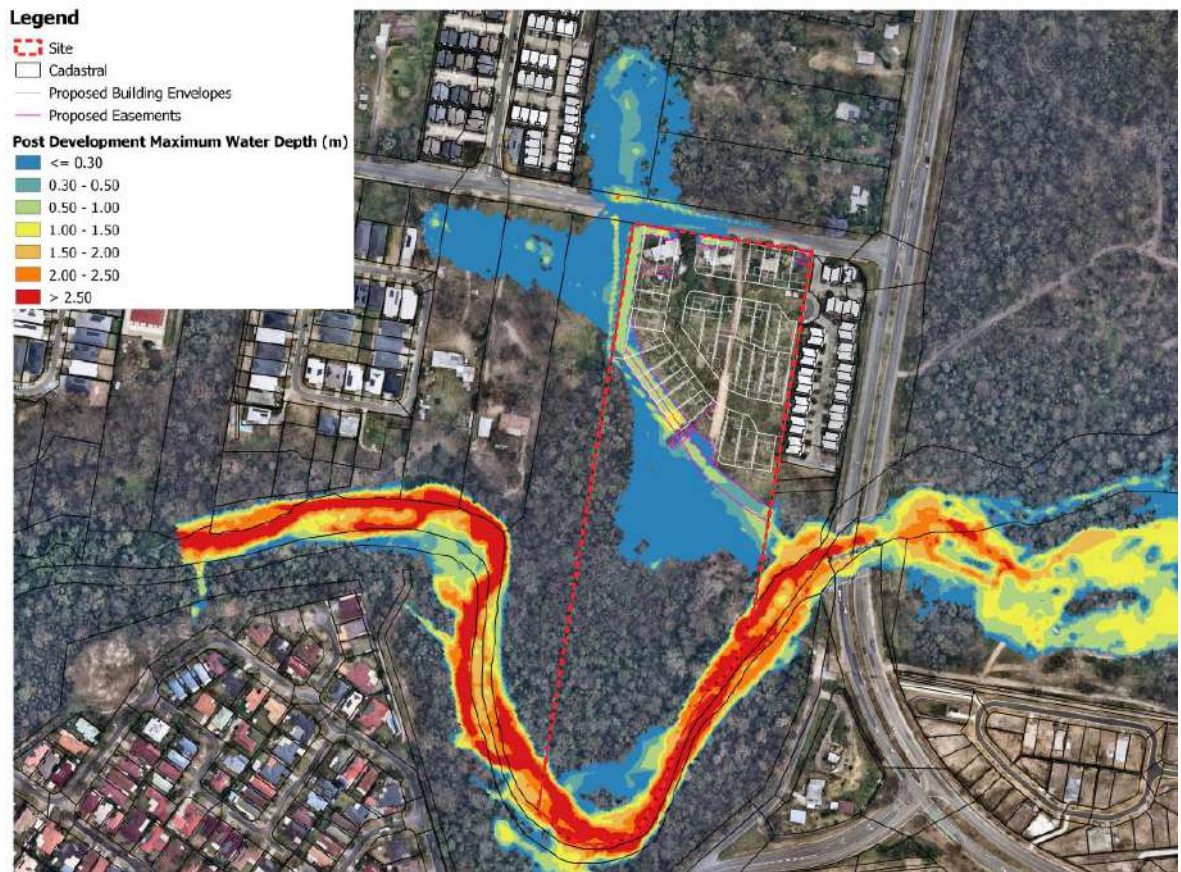
Figure 11: 2% AEP Post Development Flood Depths
