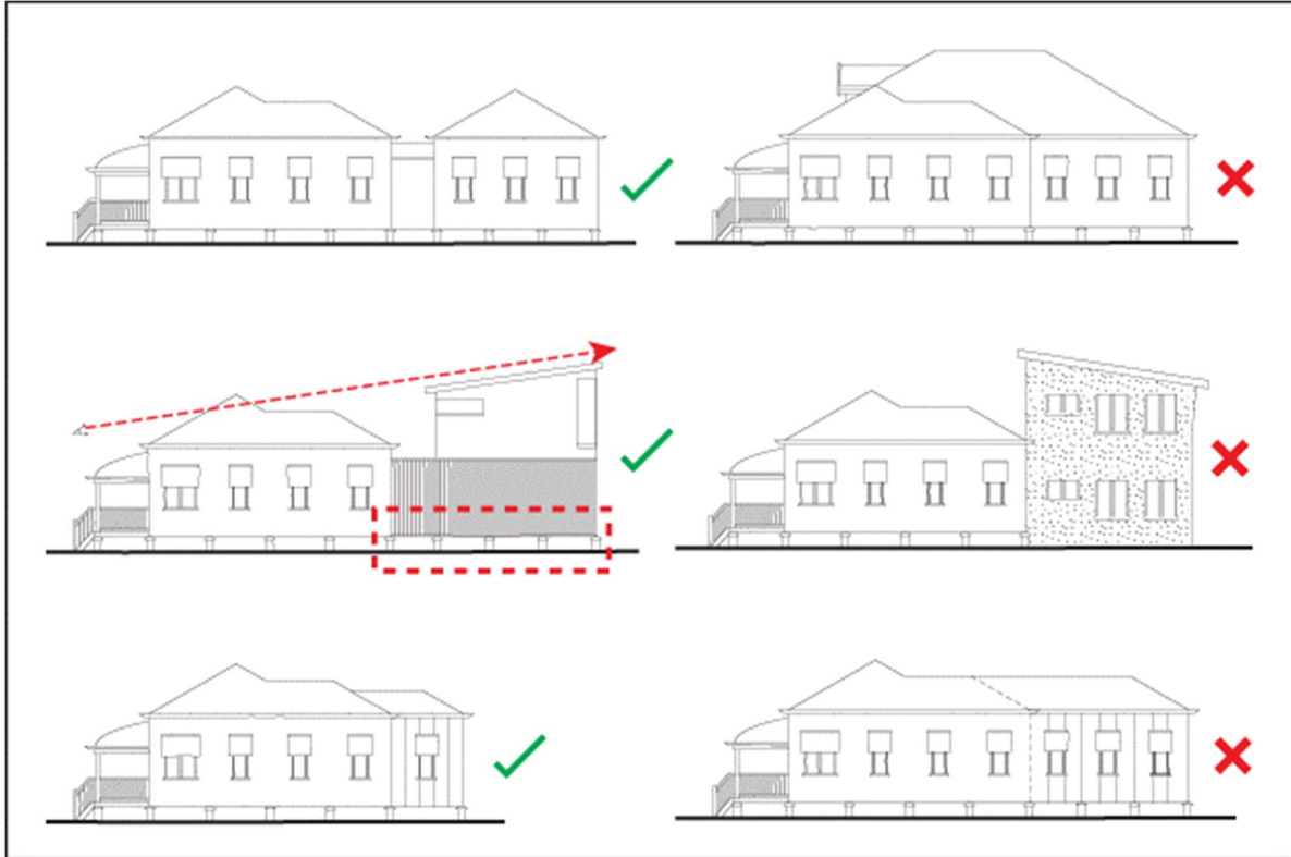
Figure f—Extensions are smaller in scale and bulk than the existing character house and generally in the form of pavilion
