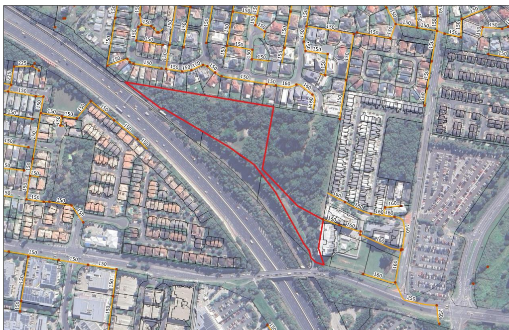
Figure 5-1 – Existing Sewer Reticulation Main (QLD Urban Utilities)
