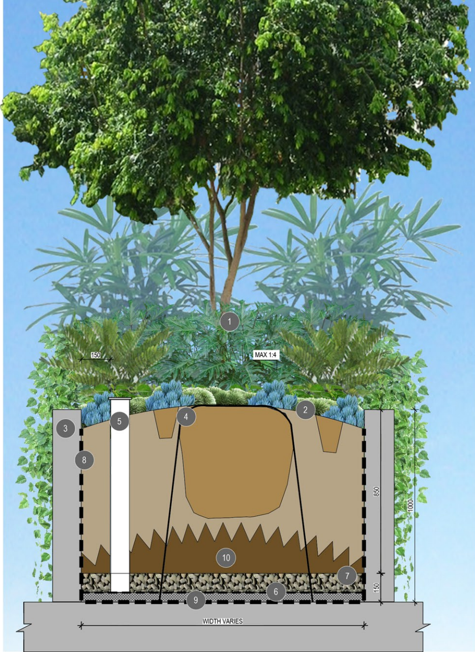
TYPICAL TREE IN PODIUM DETAIL (MIN. 1000mm DEEP) SCALE 1:10
